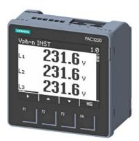
SENTRON PAC3220 LCD 96X96 mm Power Monitoring Device Controll panel instrument for electrical values protocol: Modbus TCP with graphics display U rated input: 690/400V 45-65Hz IE rated input: X/1A oder X/5A AC Power supply: 100 ... 250 V +-10 % AC/DC screw connections
